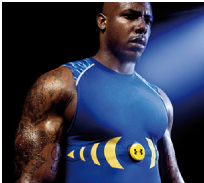
Under armour E39 compression shirt with embedded Zephyr Physiological Status Monitor 26
